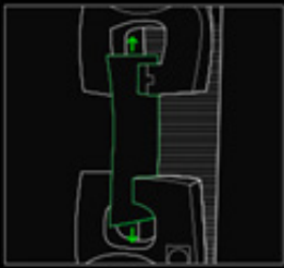
>50lbs tensile strength pulling test
