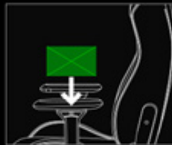
235lbs vertical force armrest test
